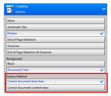
Configurations in the [Normal dialog] can be saved to a profile so that you can select a different [Deskew Method] for each document.
